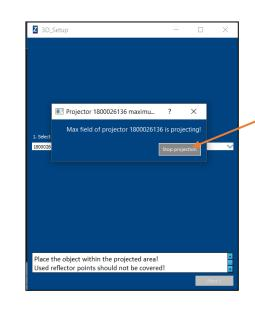
Then the max. field is projecting, the area to be projected must be within the max. field. If that is guaranteed stop projection by pressing the button: "Stop projection"
